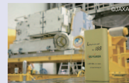
A lithium-ion cell made by GS Yuasa Technology for the International Space Station, with a cargo pallet holding the station's new batteries in the background
